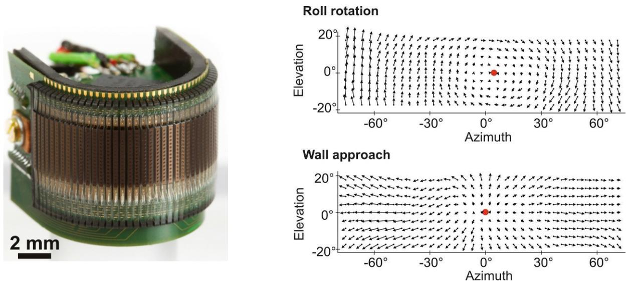
**Figure 1.** Left, image of a semi-cylindrical CURVACE prototype. Right, extracted optic flow maps across the field of view of the CURVACE prototype during roll rotation (top) and translation towards a wall (bottom). The red circles mark the center of rotation and the focus of expansion, respectively.
